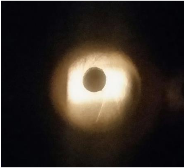
Good: Band of light correctly over the iris hole.
