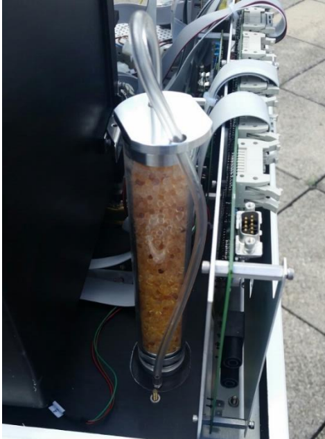
Double Brewer desiccant tube location and instructions on how to remove it.
