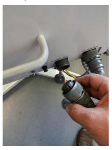
3. Use the connector plug to cap the tracker data cable to prevent moisture entry into the tracker data cable and use the Brewer data cap to cover the data bulkhead on the Brewer. This will protect the threads and keep the contacts clean and dry.
