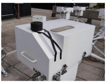
2. Remove the Brewer cover. Manually rotate the zenith prism down to the lamps by turning the brass combination gear mated to the small motor gear.
