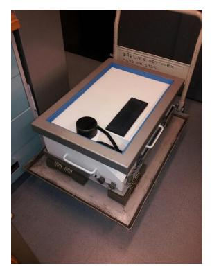
Place one strap around the Brewer length-wise and the other width-wise to secure the Brewer between the frames. Secure straps at the strap buckles and place foam between buckles and lid to protect lid from rubbing buckles.
