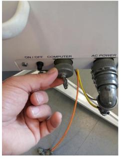
Repeat these steps for the Azimuth cable next and finally the Power cable.
