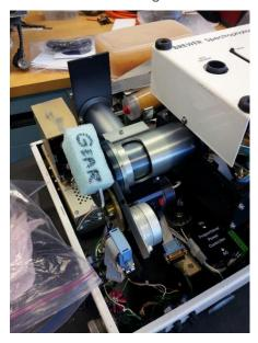
4. Insert the piece of foam labelled "Under Spec. Housing", between the spectrometer case and case base or the heat sink assembly if it is an older single Brewer.
