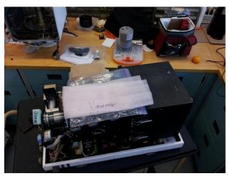
6. Use elastics to ensure the container of desiccant inside the instrument cannot open during shipping. Also secure the desiccant tray in place with elastics or cable ties to ensure the tray cannot move around during shipping. Replace the Brewer cover
