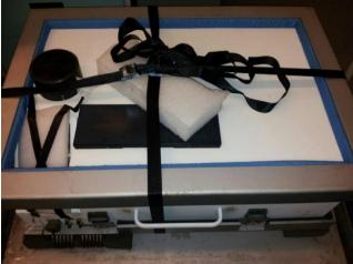
Place duct tape over each one of the packing case latches to prevent them from being torn off during shipping (latches sometimes release when the packing case is compressed).
