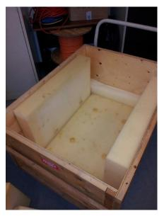
Place Brewer into the shipping crate. Place the Shipping instructions on top of the Brewer. Replace the sides and top piece of foam. Screw the plywood lid back on.
