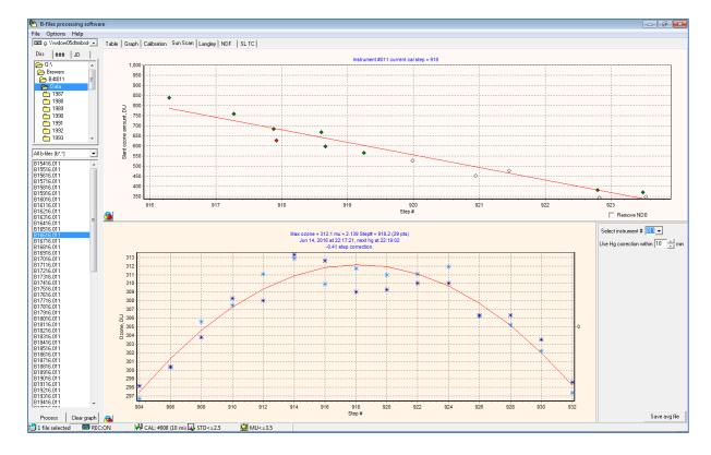
13. After validating the sun scans to be used in the slant ozone calibration line the plot may look like the following.
